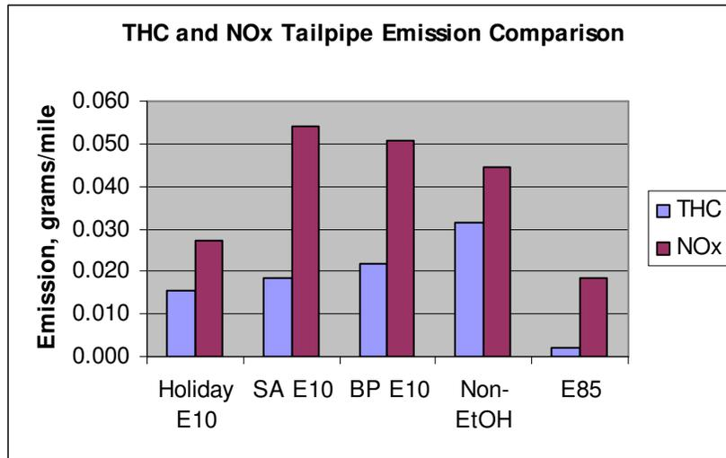
Figure 1. Comparison of fuels based on THC and NO<sub>x</sub> tailpipe emissions from 2004 E85-capable Ford Explorer operated on 505-second-duration hot-start portion of EPA FTP-75 driving cycle.
