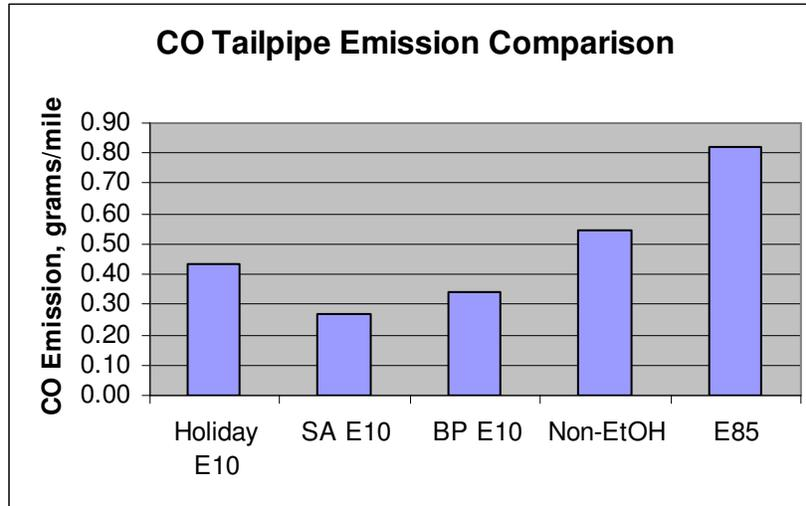
Figure 2. Comparison of fuels based on CO tailpipe emission from 2004 E85-capable Ford Explorer operated on 505-second-duration hot-start portion of EPA FTP-75 driving cycle.
